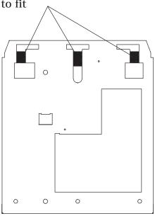
Secure unit to wall using these anchor bolt locations ,
