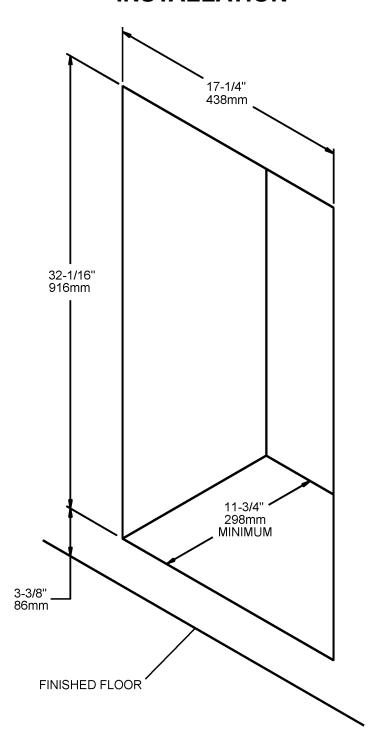
THERE ARE HOLES AND KNOCKOUTS PROVIDED ON EACH SIDE OF THE MOUNTING BOX THAT ARE INTENDED TO BE USED TO MOUNT THE BOX. USE SIX SCREW OR BOLTS (NOT PROVIDED)
